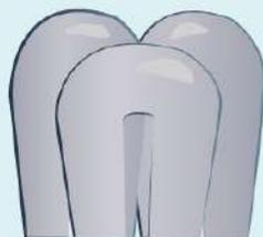
► **Step 6:** The silicon deposits onto the filament, turning it into a thick rod that is at least 99.9999% silicon.
